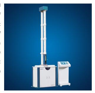
The maximum value acceptable for the TIR is taken to be 10%. There are two test methods-round-the-clock method and staircase method.
