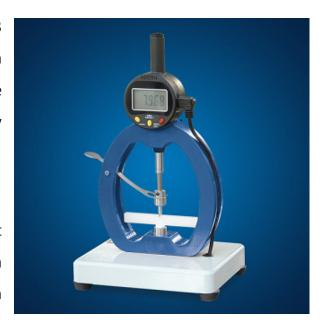
Connected to PC enables the following functions: collect the specimen width, specimen thickness, as well as the residual thickness of specimens. Put the absorbed impact energy into application software and SW will calculate the impact strength.
