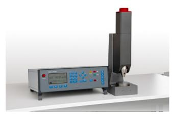
The Brinell-machines use a modified procedure to scale the penetration, since the optical measuring of the indentation isn't useful in a fast, automated testing. The test load is regulated and scaled steadily during the load application. The result is a high accuracy with a fast measuring speed.
