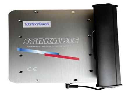
SYNKABLE video extensometer adopts Digital Image Correlation (DIC) technologies, it is a contactless method to measure elongation/Extension/deformation/deflection (strain). Video extensometer can track down the test from the beginning, this makes the calculation of elongation at break from software becomes available.
